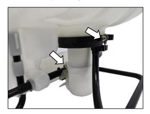
3. Unscrew the socket cap screw on the pump handle stop and remove the stop
