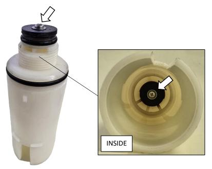
c. **Inspect the Diaphragm and valves**: Check all rubber sealing components for signs of wear, damage or cracking.
