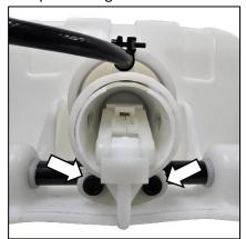
6. Carefully remove the diaphragm pump from the tank assembly.
