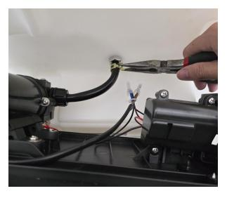
f. Once the spring clip is squeezed and hose removed from tank fitting, the cover should lift away easily.
