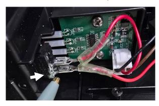
C. Ensure the battery is **not** inserted and the power switch is in ON position. Switch the multimeter to <u>resistance mode</u> ( $\Omega$ ) and touch the probes to the terminals, as shown below. If the multimeter shows no reading or remains "OL", the power switch may be damaged and should be replaced.
