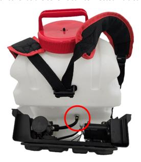
e. Locate the suction hose connecting the pump to the tank and squeeze the spring clip.
