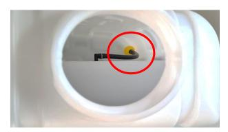
b. Gun filter, ensure the filter is securely screwed to the hose end. If not, check whether the gun filter has dislodged and is jammed in the handle blocking the flow.
