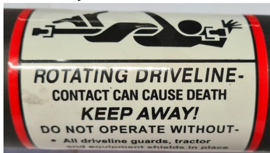
Safety Decal on PTO shaft cover
