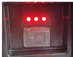
SWITCH POSITION: O = OFF, 1 = ON
