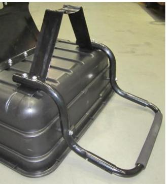
When attaching the handle fit the 2 <u>plastic spacers.</u>
