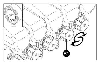
The bypass compensators are then adjusted correctly.
