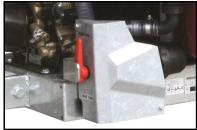
The manual pressure regulator on the discharge side of the pump is used to set the system maximum pressure, which is set higher than that required for spraying to ensure correct operation of the electric pressure regulator. Excess fluid from the pump is by-passed through the manual regulator and the electric pressure regulator back to the tank and helps keep the contents agitated.
