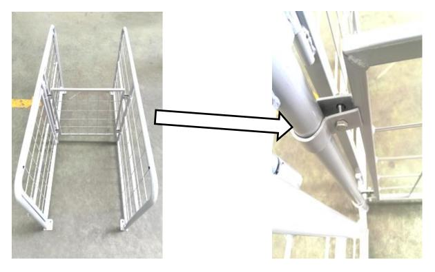
**Step 2.**Attach left and right fences, (C) & (F), using M8x50 bolt (4) as shown. Use 4 bolts per side.
