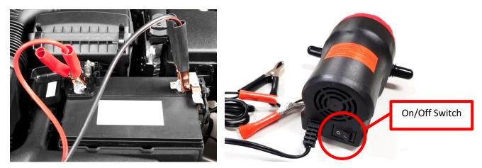
4. For best results change the oil on the engine while the engine is still warm. This helps to remove all the contaminents and warm oil will flow faster and more easily through the oil change pump.
