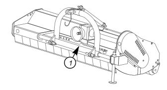
Grease rotor bearings (1).
