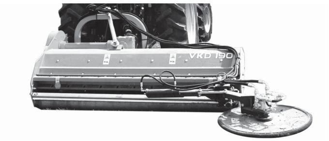
Machine with hydraulic power unit
