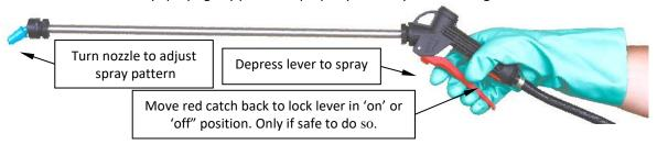
After spraying is completed, drain unused chemicals from the tank. Rinse the tank with clean water then operate the sprayer with clean water in the tank to clean out the pump, hose and spray lance. Do not leave chemicals in the tank as they may crystallize or form solids in the pump, spray lines and block the filter.
