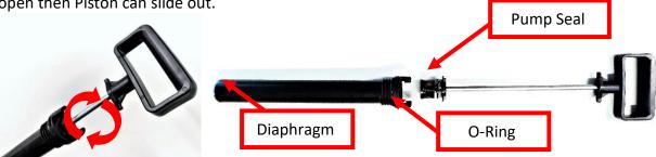
Inspect under the diaphragm for dirt or debris and clean. Remove diaphragm and clear; replace if damaged. Check pump seal is clean and lubricated (Vaseline/Petroleum Jelly).
