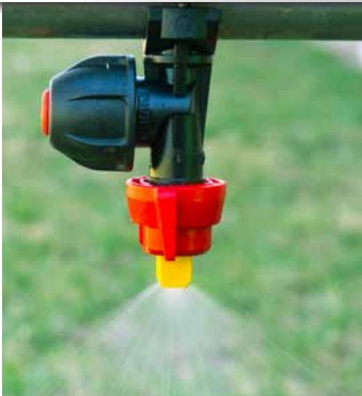
Flat spray tips have finely crafted thin edges around the orifice to control the spray. Even the slightest damage from improper cleaning can cause both an increased flow rate and poor spray distribution. Be sure to use adequate strainers in your spray system to minimize clogging.
