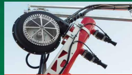
High performance hydraulic drive centrifugal fans are engineered to provide the high air velocity for optimum spray coverage
