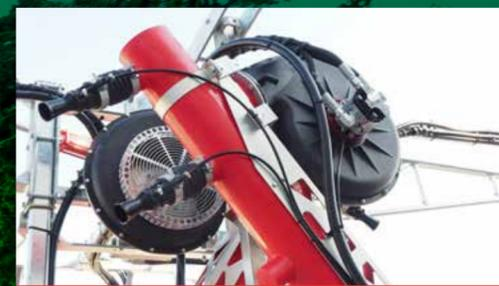
Fan hydraulic motor is isolated from the airstream meaning no chance of oil contamination if seals are compromised
