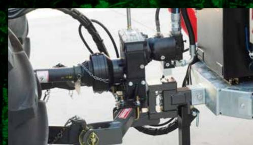
Hitch mounted hydraulic powerpack means PTO is protected and maneuverability is increased
