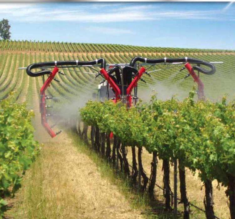
Silvan's Turbomiser sprayers have been developed to save time and money with air shear technology which uses up to 65% less water compared to dilute sprayers. They incorporate curved air tubes and adjustable swivelling heads to accommodate various canopy shapes. All Turbomiser over row sprayers feature independent nozzle rate control for target spraying. Automatic spray rate controllers are standard for precise application rate control.
