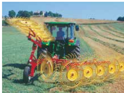
Pictured: QR Hayrake with left arm hydraulically folded
