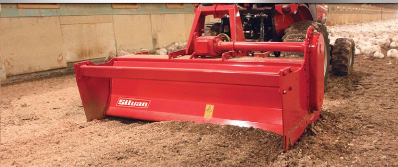
Following the introduction of new animal welfare regulations relating to the poultry industry, Silvan have specifically developed the Silvan Poultry Litter Rejuvenator (PLR) Rotary Hoe.
