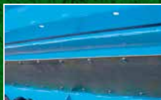
Double skin or wear plate options for increased working life
