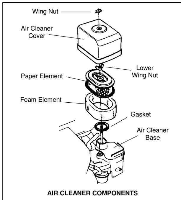
Unscrew the wing nut and remove the air cleaner cover. Unscrew the lower wing nut and remove the filter assembly. Remove the outer foam element from the paper element.
