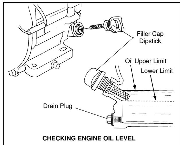
Running the engine with a low oil level can cause serious damage. To safeguard against this the engine is fitted with a 'low oil level' protection system that automatically stops the engine if the oil drops below the safety level. When this occurs the ignition switch remains in the 'on' position. If the engine should stop during operation always first check the oil level before looking for other causes.
