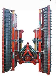
Comes with cage or packer roller options for better soil compaction, levelling and seed bed preparation
