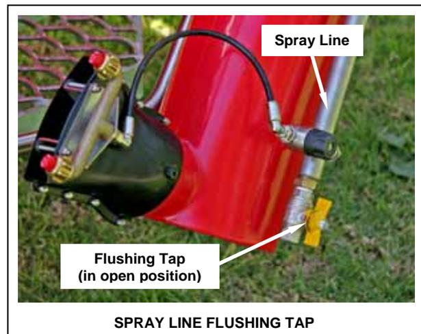
Add clean water to the tank and run the sprayer at 540 PTO rpm for several minutes with all sections open to flush the system and remove all chemical from the pump, valves and spray lines.
