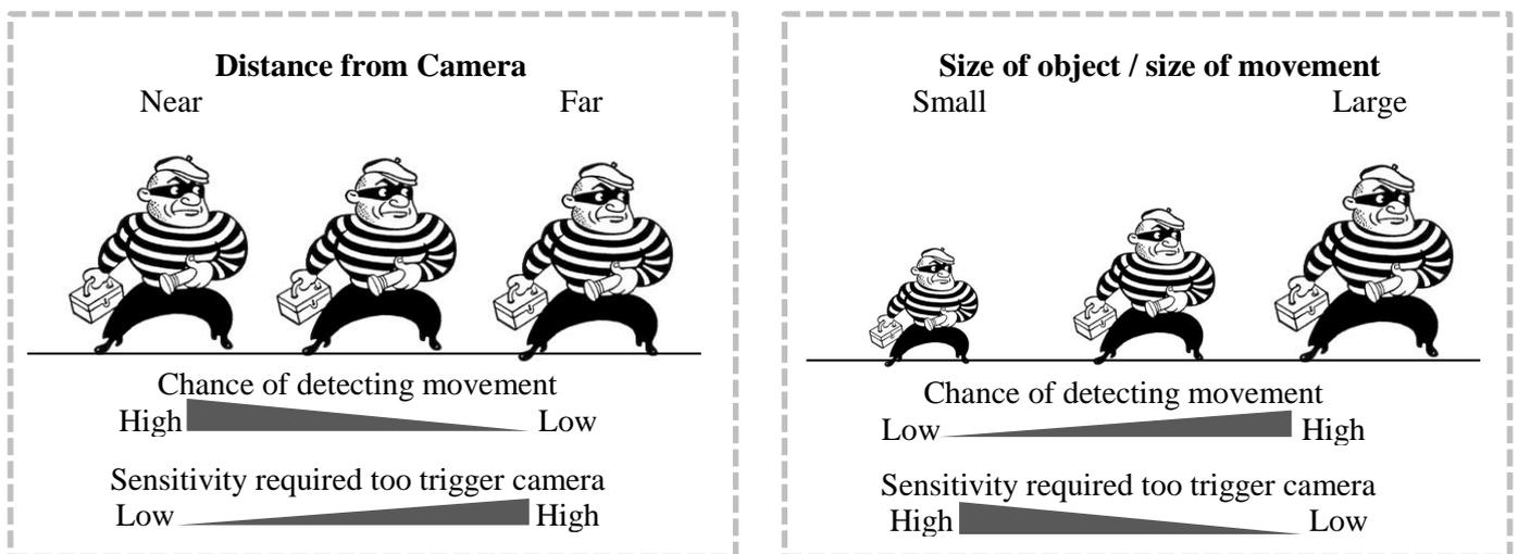
For interior areas and environments with little interference, such as branches blowing in the wind, select "High". Select "Normal" for exterior areas and environments with a normal amount of interference, and select "Low" for environments with a high level of interference. The temperature can also affect the sensitivity. The "High" setting is suitable for warm ambient temperatures, whereas "Low" should be selected for cold environments.
