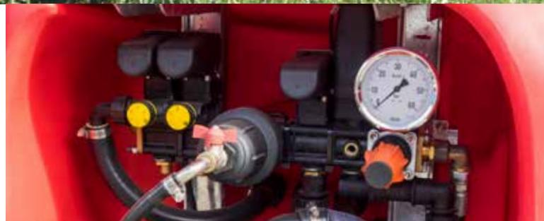
All Silvan trailed orchard sprayers are fitted with modular electric valves that provide greater control of sprayer output. They offer independent left and right section control along with pressure adjustment from the tractor cab.
