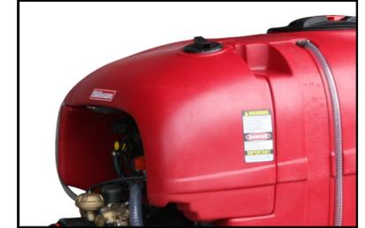
The level of liquid in the main tank is shown by either the front or side sightlines on the sprayer. The flush tank can be filled through the locking cap at the front of the tank. To use the flush tank to clean the pump, filters, spray lines and nozzles the suction valve is turned to Flush Tank and the sprayer is operated as outlined in following pages.
