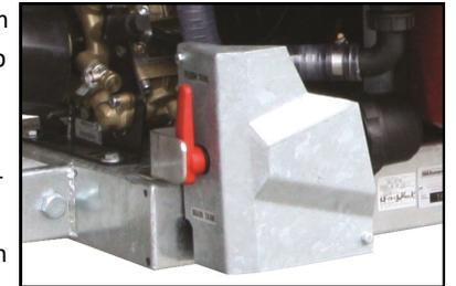
The manual pressure regulator on the discharge side of the pump is used to set the system maximum pressure, which is set higher than that required for spraying to ensure correct operation of the electric pressure regulator. Excess fluid from the pump is by-passed through the manual regulator and the electric pressure regulator back to the tank and helps keep the contents agitated.
