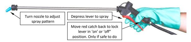
After spraying is completed, drain unused chemicals from the tank. Rinse the tank with clean water then operate the sprayer with clean water in the tank to clean out the pump, hose and spray lance. Do not leave chemicals in the tank as they may settle and form solids that may block the filter.
