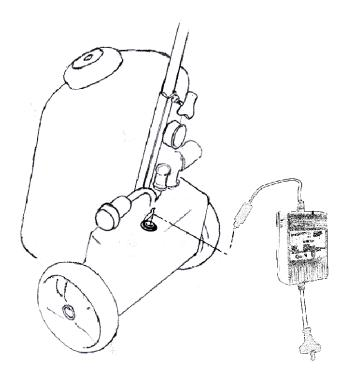
Ensure that the TrolleyPak's power on/off switch is set to off. To charge the battery, connect the plug of the charger to the socket located at the rear of the sprayer as shown in the diagram above and turn the power on the charger.
